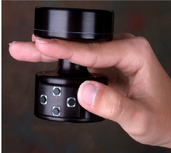
Figure 2. NIS depicted with four-button thumb control. The acoustic mode “on” switch is located at the top, and Doppler mode “on” switch is at the bottom (there is an automatic timed shut-off). Volume increase and decrease switches are located left and right, respectively.
