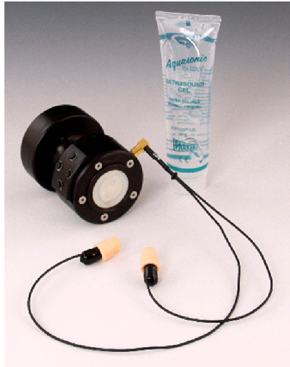
Figure 1. Noise Immune Stethoscope device depicted with Communications Ear Plugs (CEPs) and ultrasound gel.
